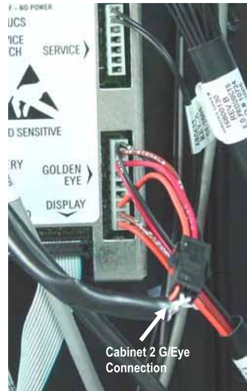
Photo 1 – Á LA CARTE Golden Eye connection in a host SNACK machine
