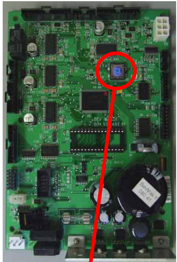
Figure 9: Location of the Service Switch
